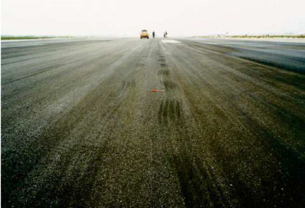
Figure 3.8: Shimmy phenomenon (from [Besselink, 2000])
